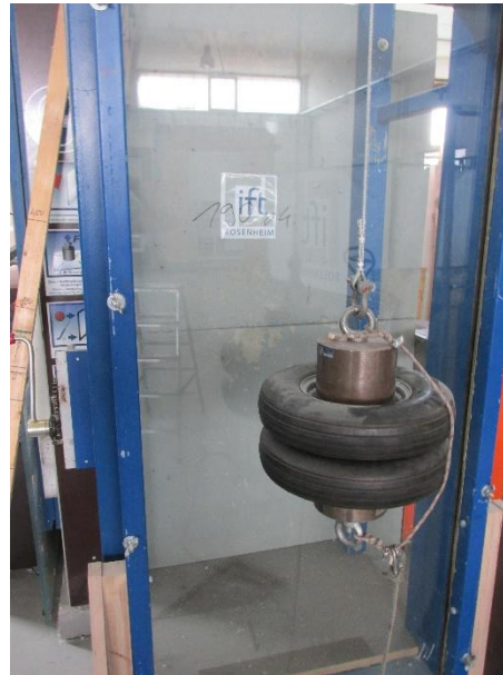
Picture 4 Test sample after 190 mm drop height
