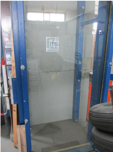
Picture 3 Sample before the pendulum impact
