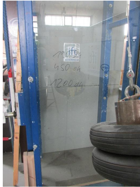
Picture 6 Test sample after 1200 mm drop height
