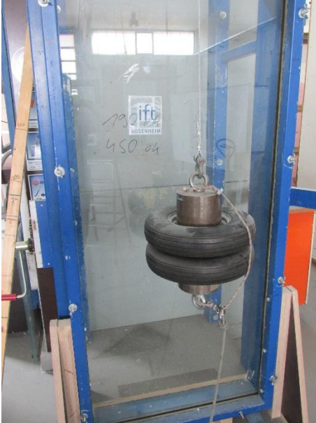
Picture 5 Test sample after 450 mm drop height
